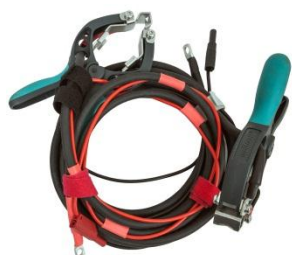
Current cables and Sense cables with TTA clamps (combined)
