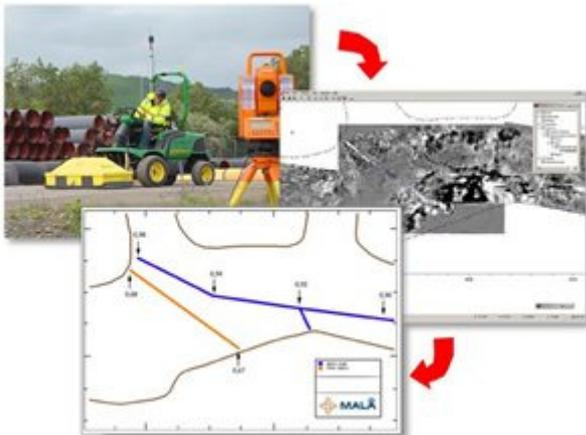
The power within this product lies in its ability to quickly and easily gather full 3D data in broad paths, so called "swots". Results are processed in 3D, displayed and interpreted through a dedicated software package and then exported into suitable GIS or CAD data formats.
